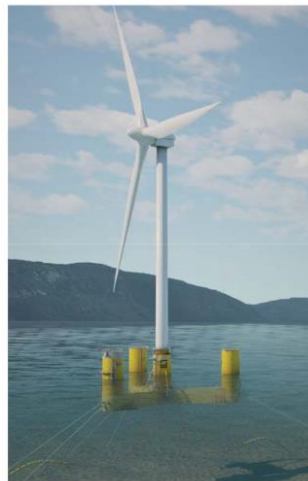
Figure 7-7 Naval Energies STAR1 floating structure design (image courtesy of Saipem)
