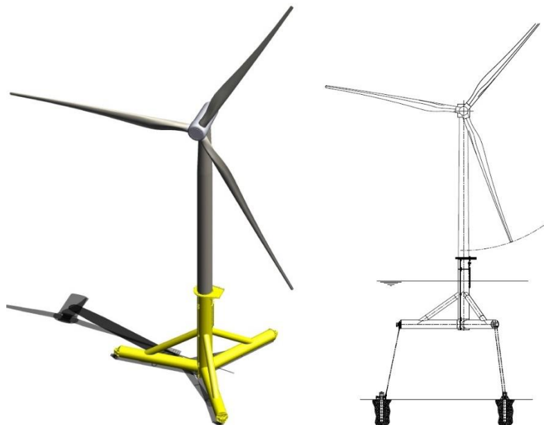
Figure 7-8 SBM TLP floating structure design (image courtesy of SBM)
